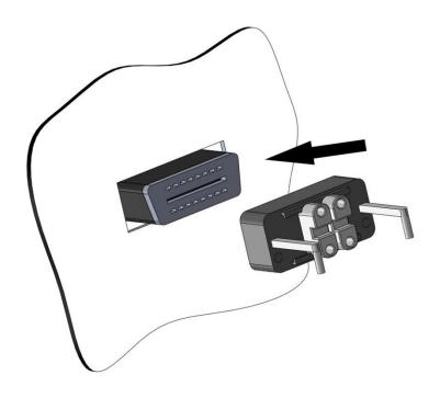
put the lower lock part onto the OBD socket jack (mounting is possible only in one specific position!)
